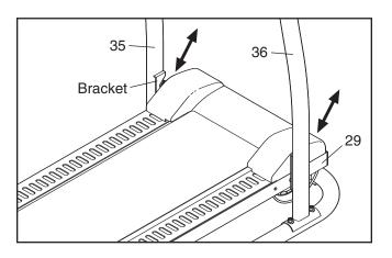
**CAUTION:** Make sure that the incline knobs are fully inserted at the same height.
